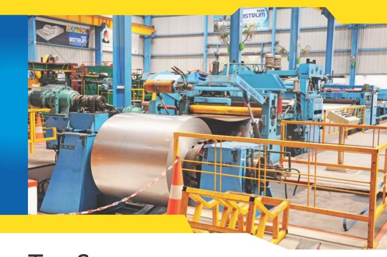
Technical Specification of CR/GP/GPSP Fully Automatic CTL (Cut-to-Length) Line 1600mm wide
